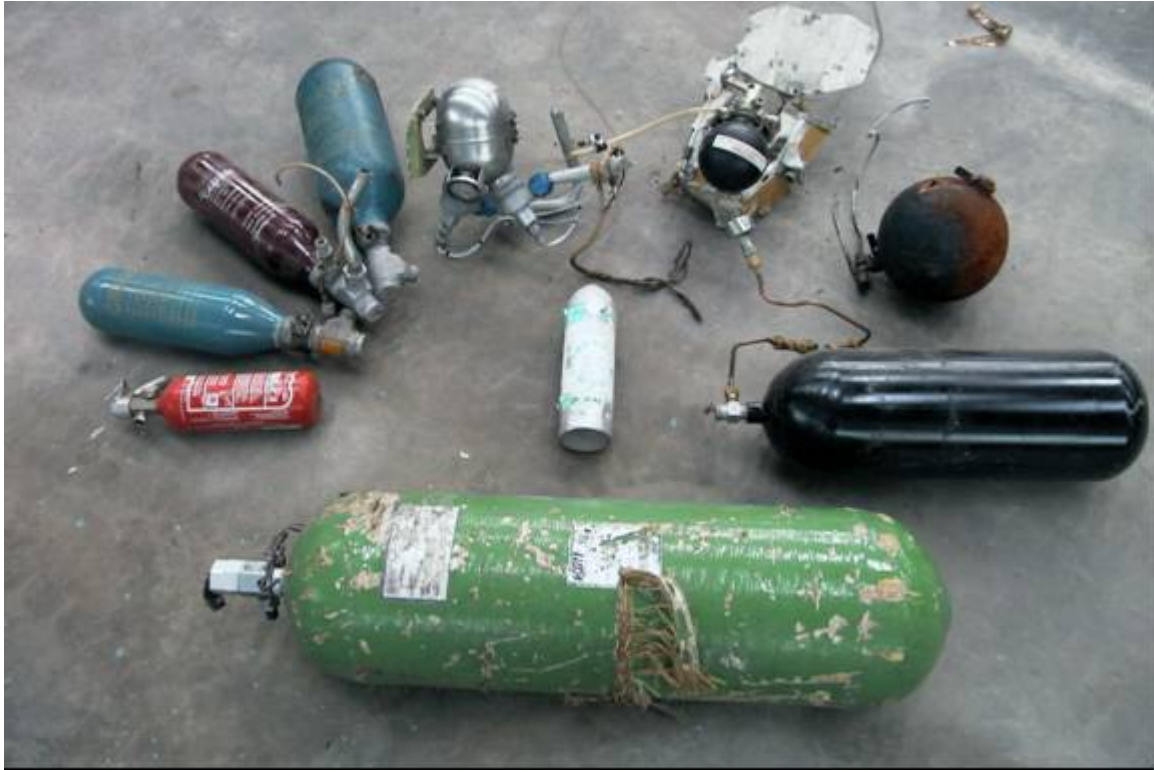
Figure 1. A selection of pressurized containers recovered from aircraft accidents
